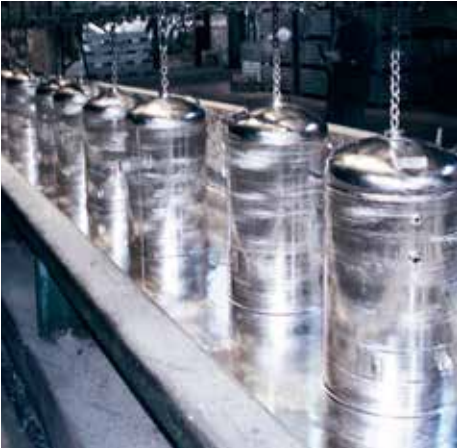
Hot-dip galvanisation for a long service life flat/upright 50 litres - 500 litres 10 bar or 15 bar
