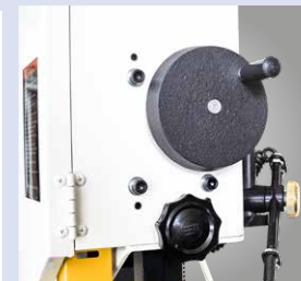
► Saw band guide height-adjustable via hand wheel
