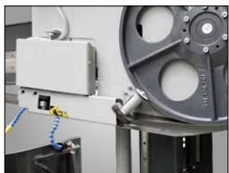
driven cleaning brush for cleaning and maintenance of the saw band
