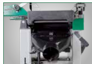
Integrated suction connection
