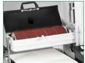
Easy and quick sanding belt replacement
