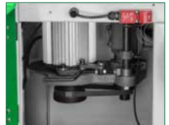
Quick and easy speed change by means of multi V-belt
