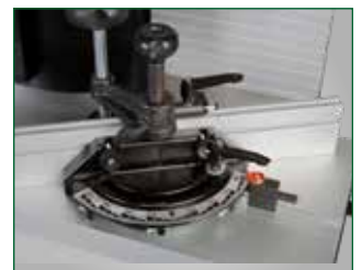
Infinitely adjustable angle stop
