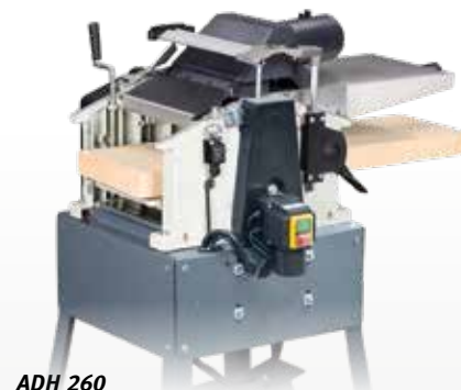
ADH 260 Converted for thicknessing
