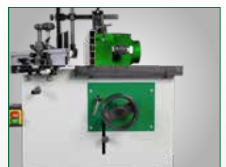
Handwheel for height adjustment. Safety devices included in the scope of delivery
