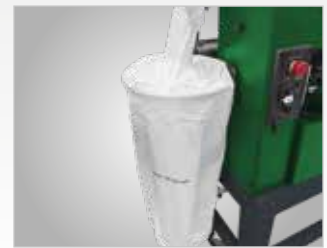
Integrated extraction system for dust-free working
