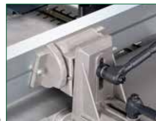
The aluminium dressing fence can be tilted by 45°. The set inclination can be easily read off a scale.
