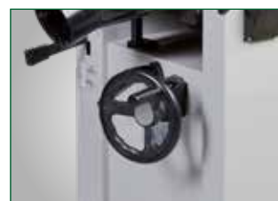
Thickness table adjustment via handwheel, scale and numerical display
