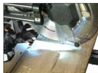
Extremely precise light projection of the cutting edge
