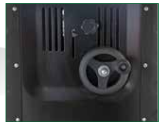
Spindle height adjustable from 0 to 40 mm
