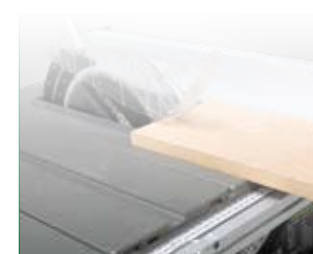
Folding rip fence for thin workpieces
