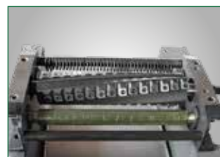
Planing unit with spiral cutterblock
