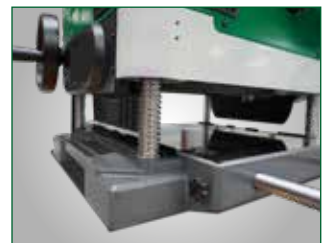
Maximum precision thanks to solid quadruple spindle guide of the planing unit
