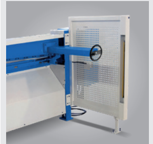
▶ Rear area secured by light barrier
