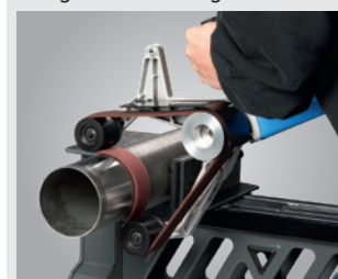
▶ Only two work steps necessary for 360° peripheral sanding
