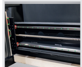
▶ The X-axis, driven by ball screws, runs on double linear guides
