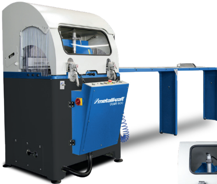
ULMS 600 with accessories Roller conveyor with length stop and manual measuring system with mm scale
