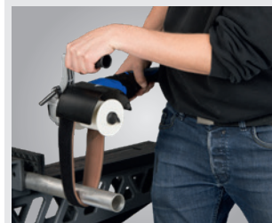
▶ Satin finishing of round steel with Velcro fleece, even with already installed stainless steel railings, for example
