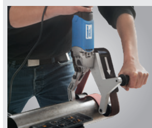
▶ Handle can be screwed in at various positions for ergonomic working
