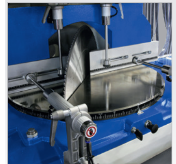
▶ Stepless adjustment of the mitre angle
