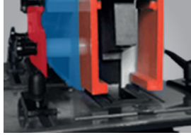
▶ Notching station (from HPS 45S)
