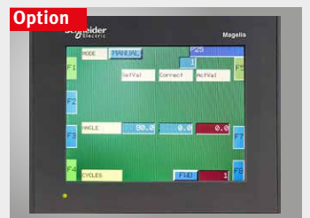
► Optional control Schneider TM 238 , single-axis control for digital angle input via generously dimensioned touchscreen with the option of storing bending sequences
