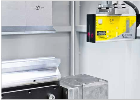
► Fiessler AKAS II safety device
