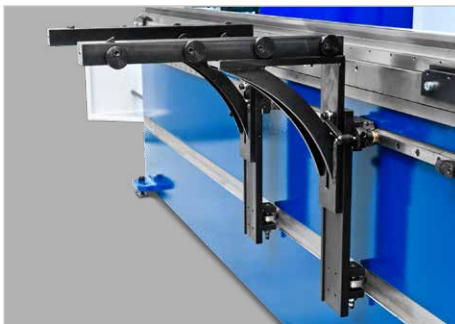
► Sheet support arms displaceable on linear rails
