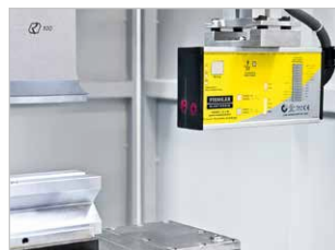
► Fiessler AKAS II safety device
