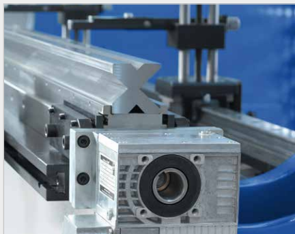
► CNC-controlled, motorised table crowning (standard for S and Servo series)
