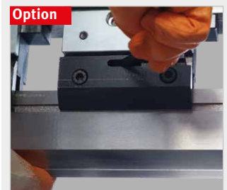
► Manual top tool quick release with cam lever (option)
