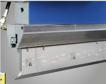
► Hydraulic top tool clamping "WILA" for easy tool changes within seconds (optional)
