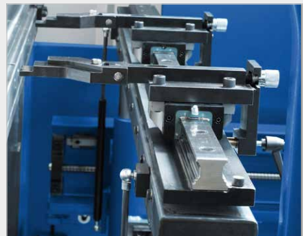
► Rear stop system with R axis (standard for S and Servo series)
