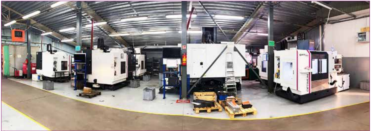
Seven F 150 CNC milling machines and two F 310HSC and one F 500HSC CNC milling machines in one of Baltec's production shops
