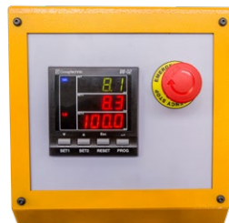
▶ Control panel with digital display and EMERGENCY STOP switch
