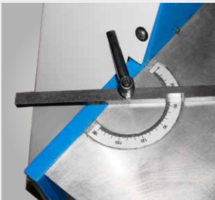
Angle-adjustable side stop with millimetre scale
