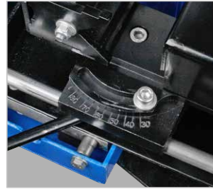
► Grinding angle of 30-90° adjustable based on scale
