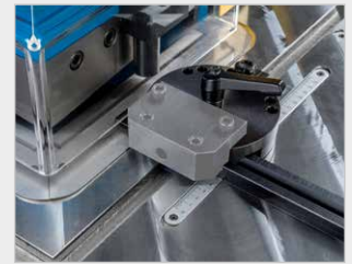
▶ Stops with adjustable blank holders
