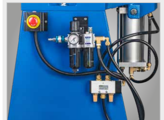
▶ Maintenance unit for pneumatics
