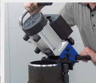
▶ Deburring of pipes possible
